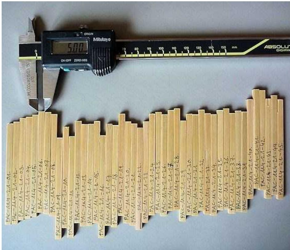
Fig. 5 Hand planed Tonkin samples for three-point-bending test, 3 mm height, 5 mm width, 80 mm length (in inches: 0.118 h., 0.197 w., 3.150 l.). Before bending each sample’s dimension and weight is measured individually.
