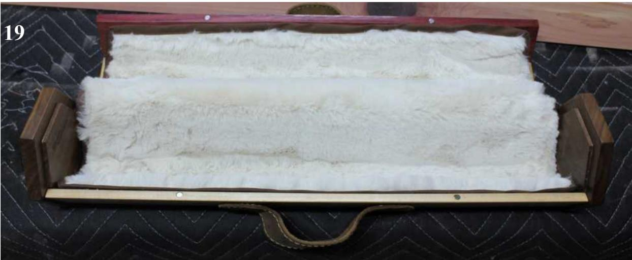
The last piece of actual woodwork that I need to do is for the end caps. I make these to mimic the hexagonal shape of the box and remove material so that they sit just inside the case body. When I'm picking wood for this, I spend time to choose something nice. I will pick a figured wood or one that is colored just right to accentuate the rest of the case features (other wood, leather, hinges, etc.) (see Photos 19, 20 and 21).
