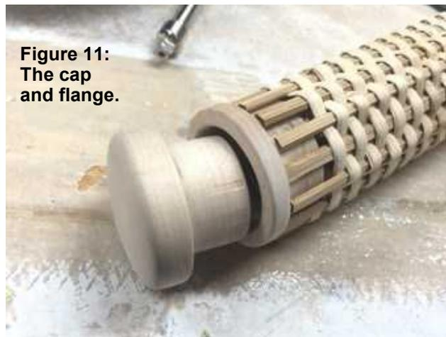
**Figure 11: The cap and flange.**
