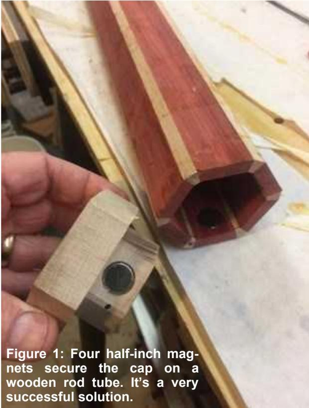
Figure 1: Four half-inch magnets secure the cap on a wooden rod tube. It's a very successful solution.
