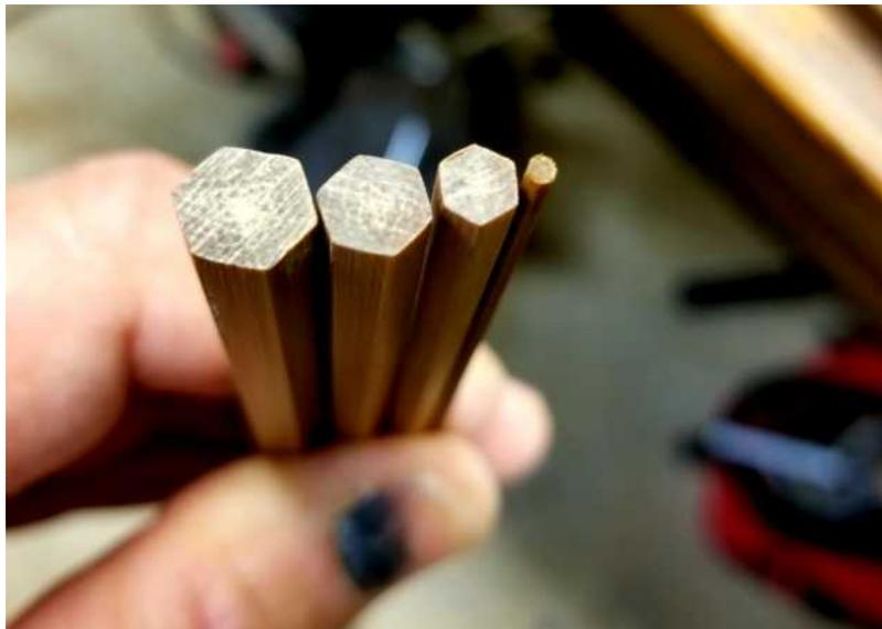
A few final points on building a splice rod, I did swell my joints 10% of the rod diameter at the center of the splice and continued the swell for the entire length of the splice. Also, it is important not to make the tip of your splice less than .040. As I stated earlier, I did hollow three sections of this rod and I made sure to stay 3.5" away from each of the splices.
