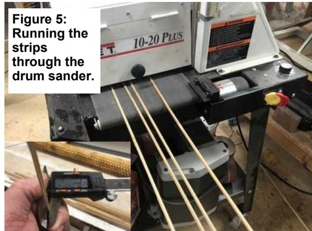
**Figure 5: Running the strips through the drum sander.**
