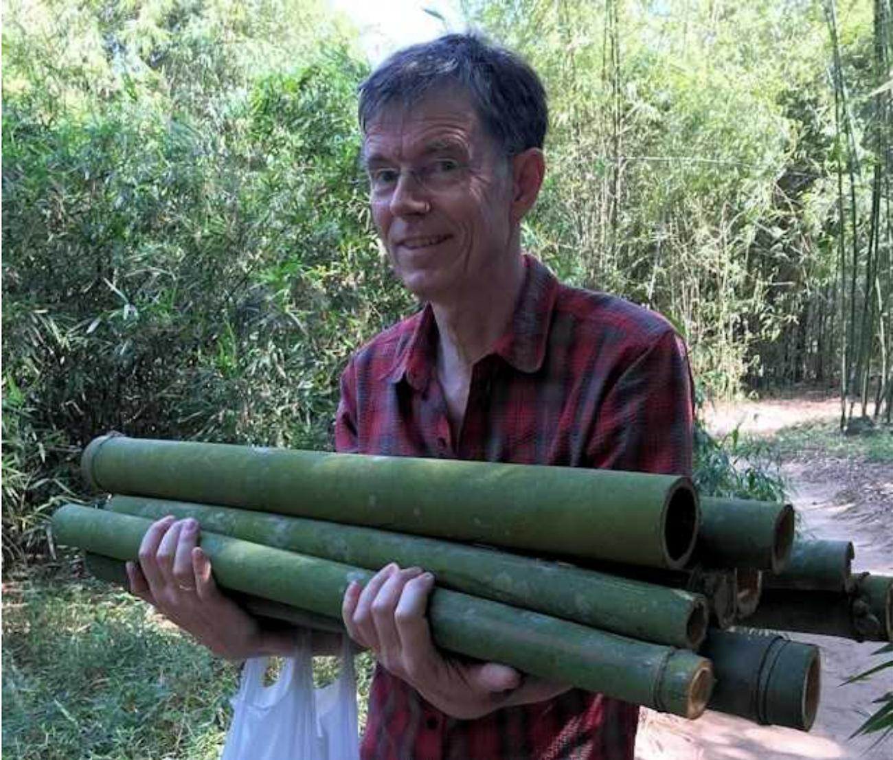
Fig. 1 Author with samples of single internodes from Viet-1 bamboo, average length 31 inch.
