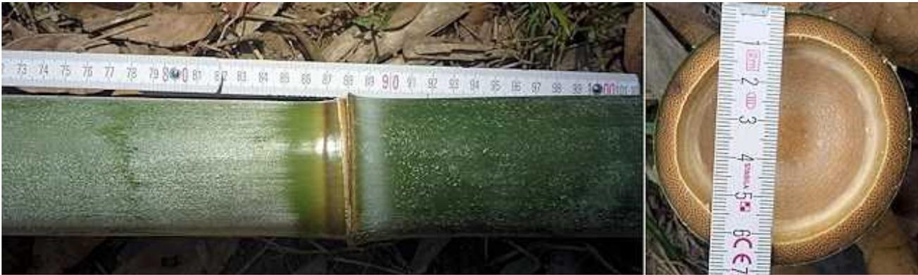
Fig. 3 Viet-2 node, internode length 35 inch, fresh-cut cross-section diameter 2.7 inch.
