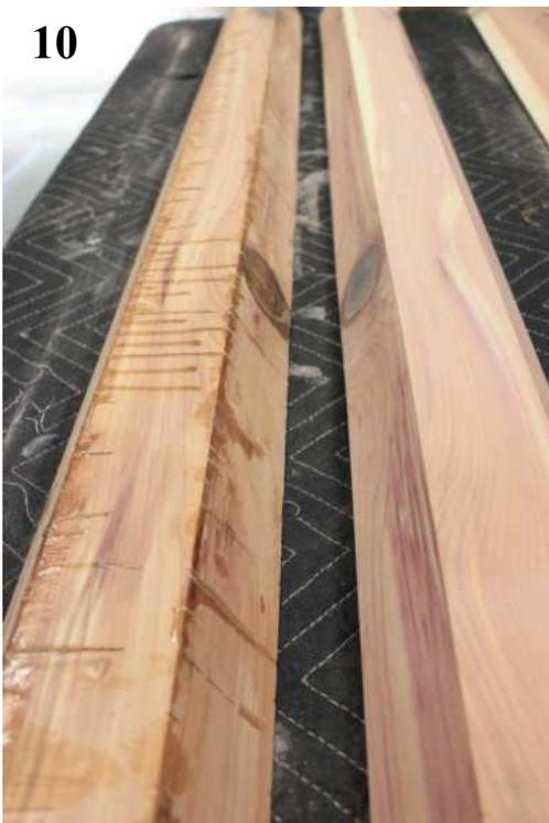
The squeeze out from the glue leaves a mess and I have to clean it up before moving along. This is the final sanding which has to get done to the full length of the box before beginning any detail work (see Photo 10).
