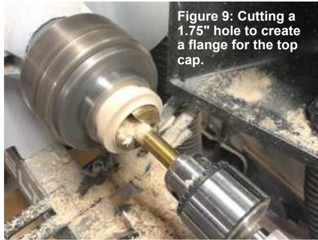
**Figure 9: Cutting a 1.75" hole to create a flange for the top cap.**
