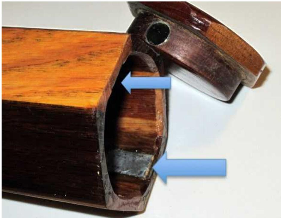
Figure 5 (Arrows denote small iron plate replacing inner magnet.)
