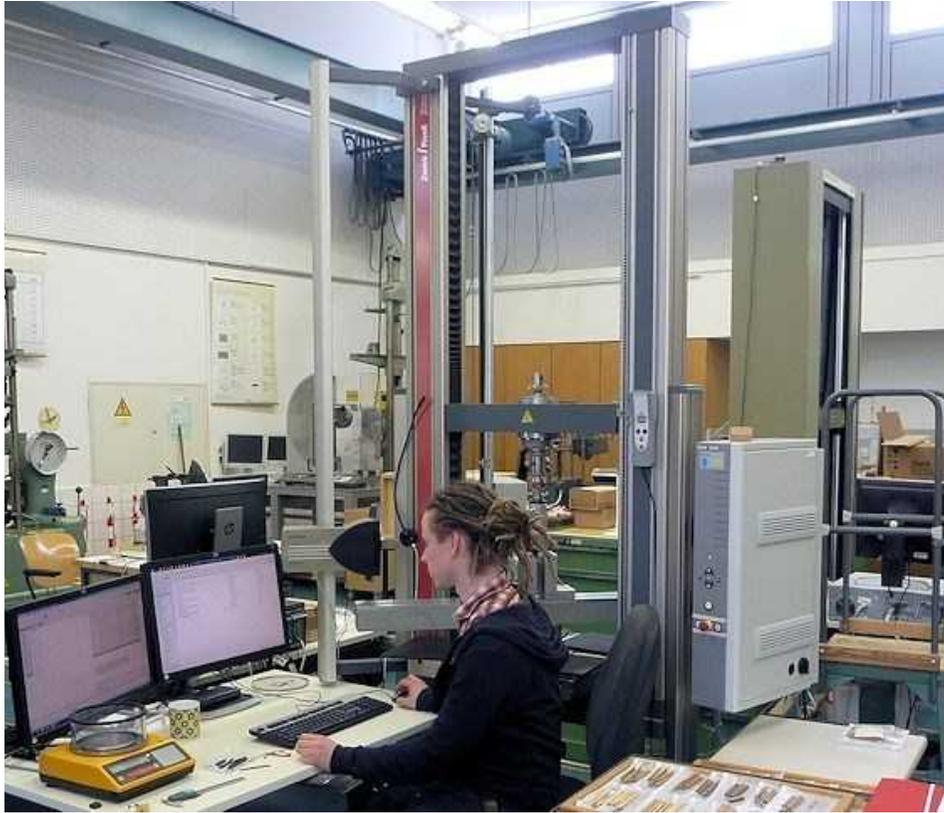
Fig. 6 Laboratory of the Institute of Wood Science, Universität Hamburg, Germany. Large three-point-bending device behind Goran Schmidt.
