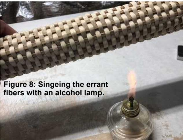
**Figure 8: Singeing the errant fibers with an alcohol lamp.**
